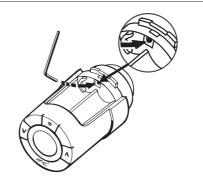
2. Insert a small hex key or similar into the locking hole to lock the adapter ring.
