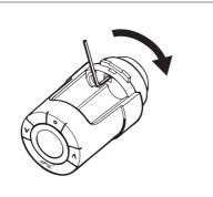
With the hex key locking the adapter ring, turn the adapter in the shown direction.
